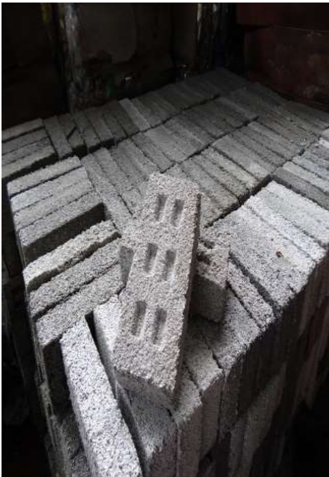
Hollow blocks using pet bottles
