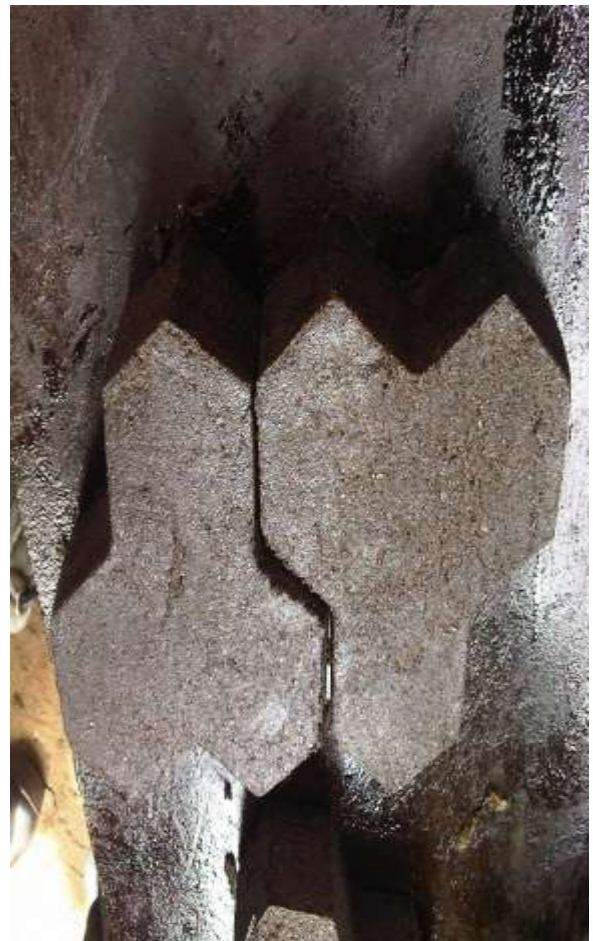
Cement Paver blocks using Scrap plastics
